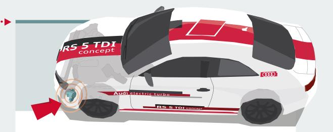
The electric V6 biturbo in the Audi RS 5 TDI concept produces 283 kW (385 hp). The electric compressor quickly provides high torque when starting off. If the driver stays on the accelerator, it takes roughly four seconds to reach 100 kilometers per hour. Boost pressure is available immediately after each gearshift thanks to the intelligent interplay between the two turbochargers and the electrically driven compressor.
